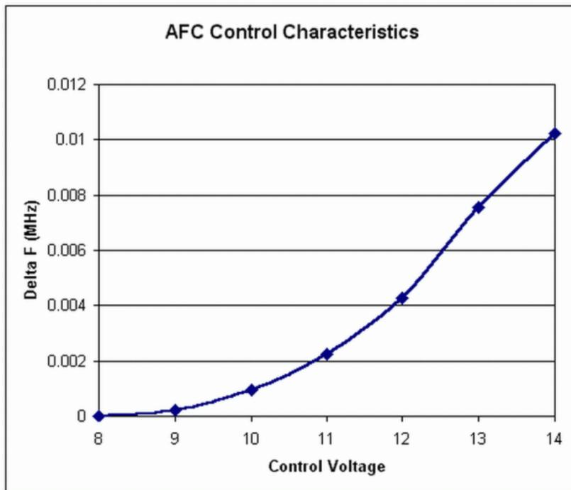
Chart of AFC control characteristics as measured.
