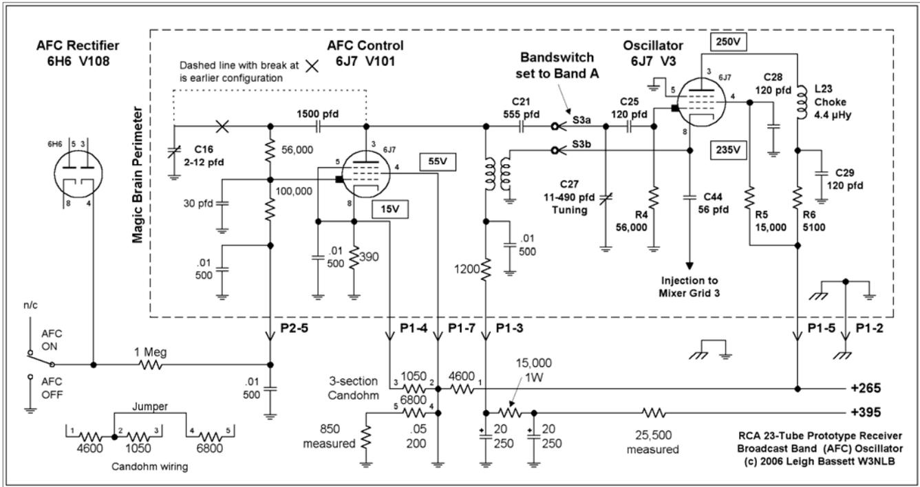
Broadcast band (AFC) oscillator schematic. Components outside the Magic Brain perimeter were measured and may not reflect the exact circuitry in the set.
