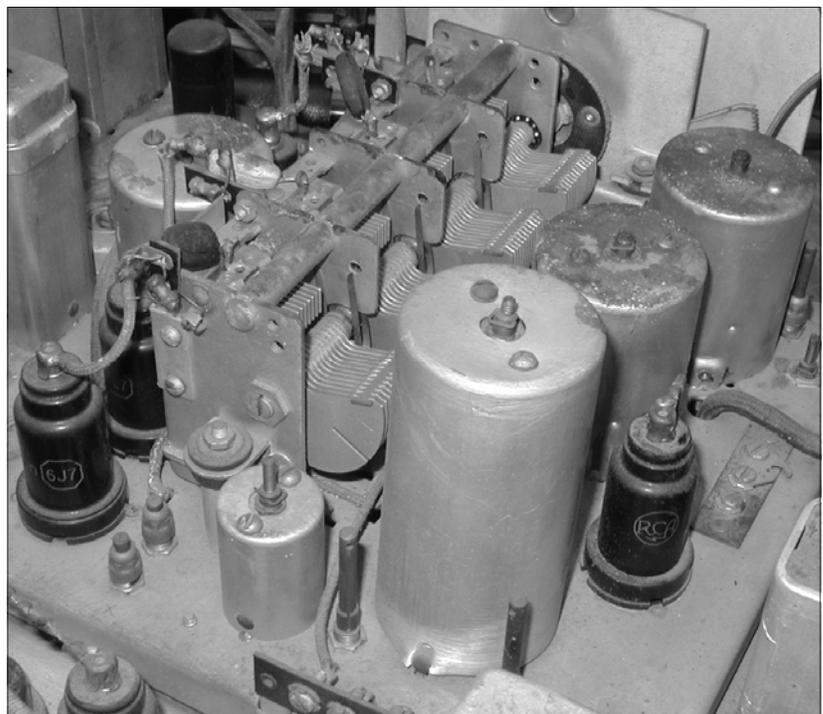
The Magic Brain section of the radio is shown here. Note the four-gang tuning capacitor.
