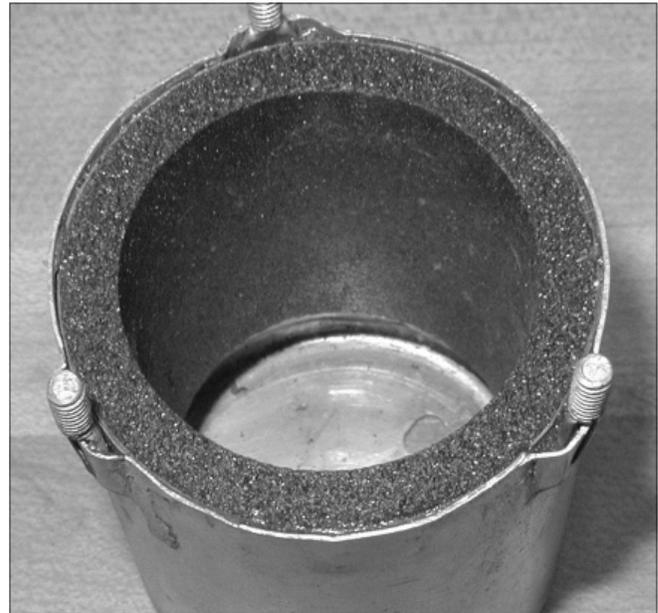
Antenna can with ferrite shield.
