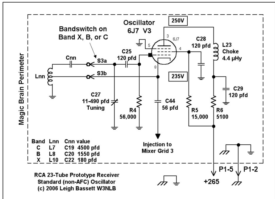
Bands X, B, and C (tapped coil) oscillator schematic.
