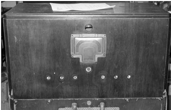
The cabinet of the prototype. The receiver portion is crudely made out of plywood, and sits atop a standard RCA speaker cabinet.
