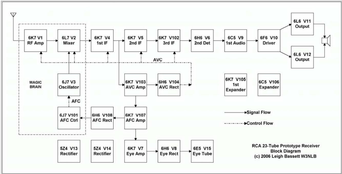
Block diagram of the prototype receiver.
