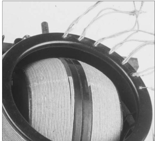
**Figure 4-7.** Detail of early variocoupler switch wiring and bifilar rotor.
