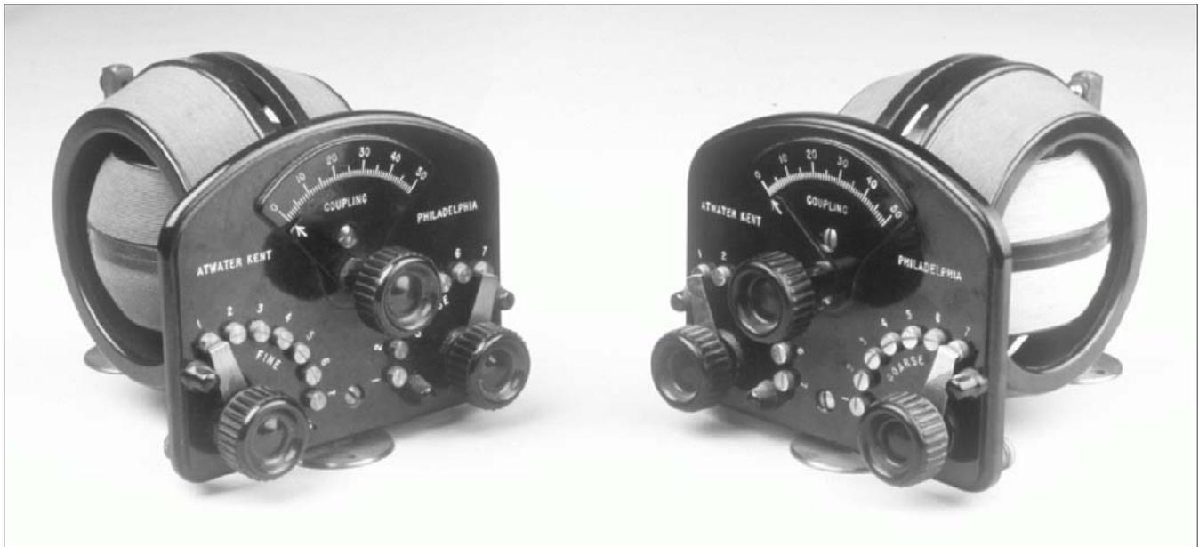
**Figure 4-4.** Mounted variocoupler # 3612 (black) or # 3734 (brown), left and right side views.
