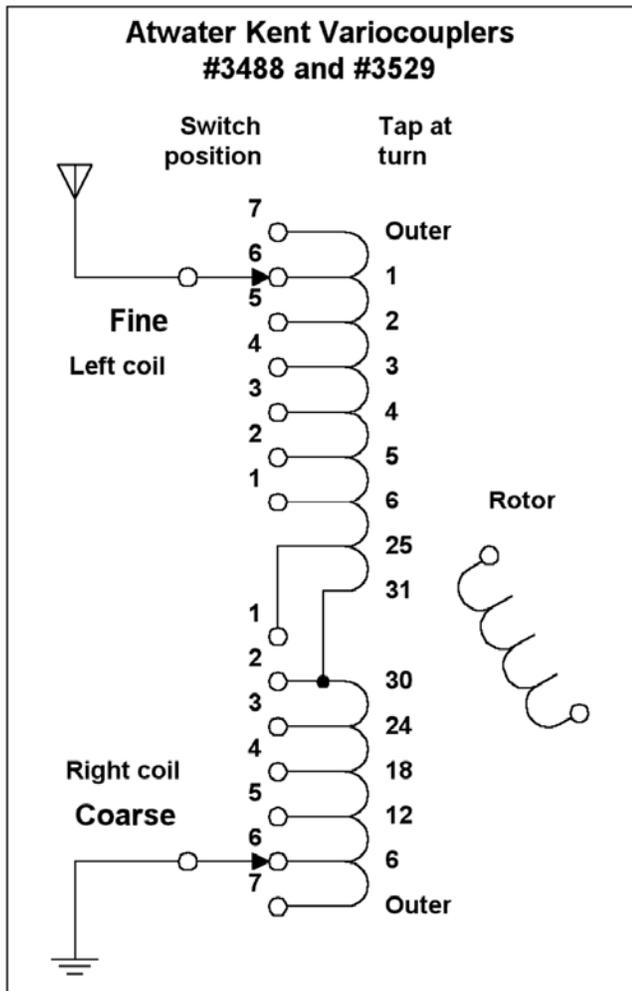
**Figure 4-6.** Schematic of variocoupler.
