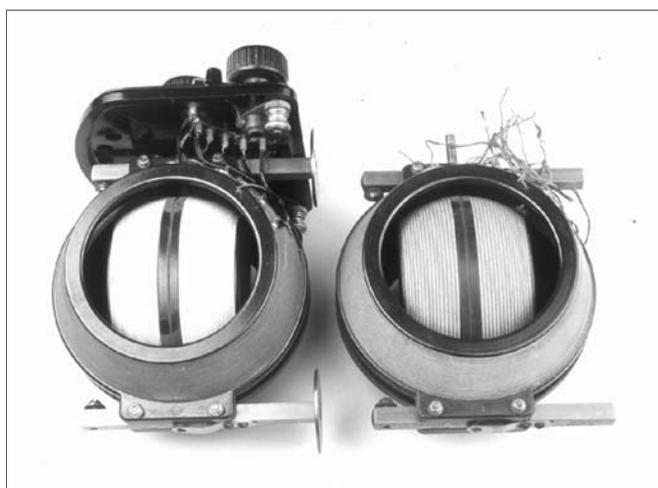
**Figure 4-8.** Left: mounted variocoupler # 3612 (black) or # 3731 (brown); Right: unmounted variocoupler # 3529 with string spacer in the rotor winding.
