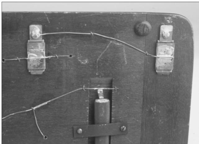
**Figure 4-15.** Antenna capacitors, bottom view.
