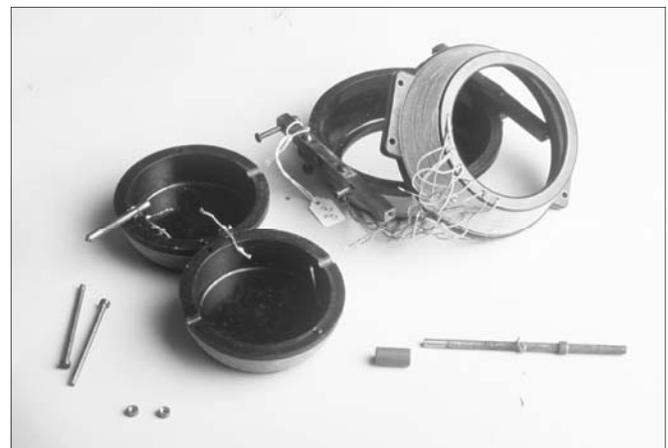
**Figure 4-5.** Disassembled early variocoupler.
